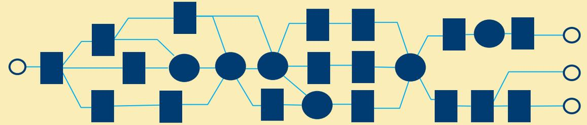
A custom hardware datapath can be generated in an FPGA for complex `single_task` kernels
