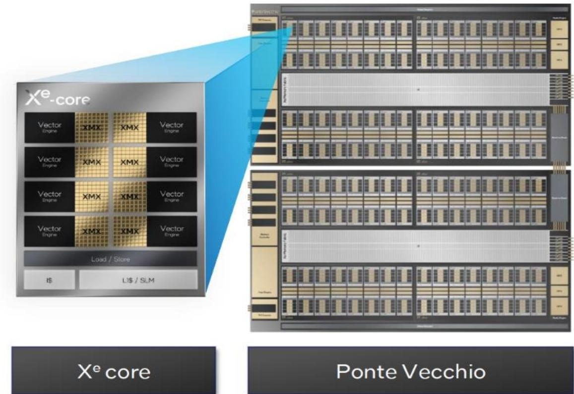
Each Xe-Stack has 4 slices with each Xe-slice contains 16 Xe-core
